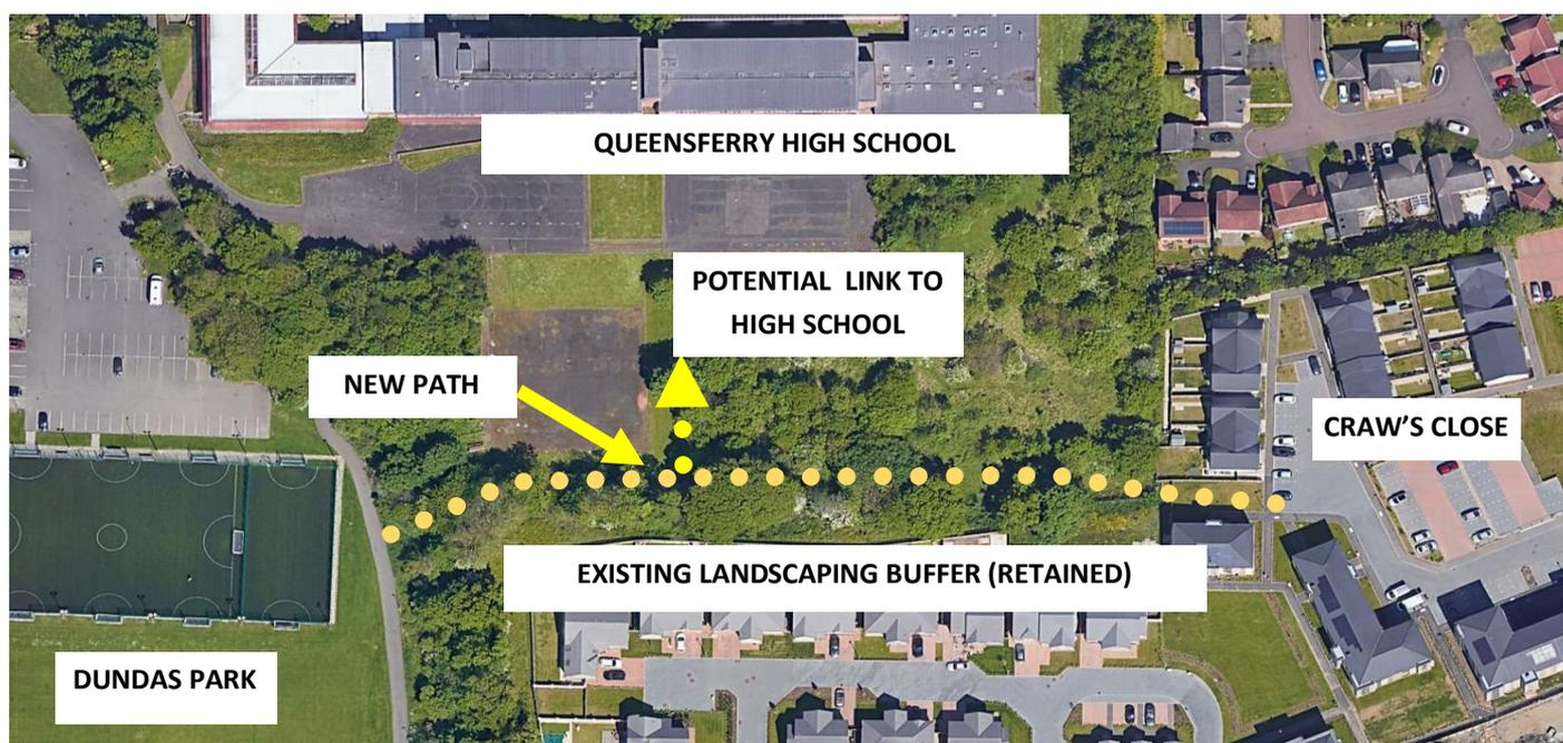
The project is looking to create a new 4m wide shared use surfaced path which, via a new ramp connection, will link the housing at Craw's Close to Dundas Park, providing an improved connection towards Queensferry High School.
